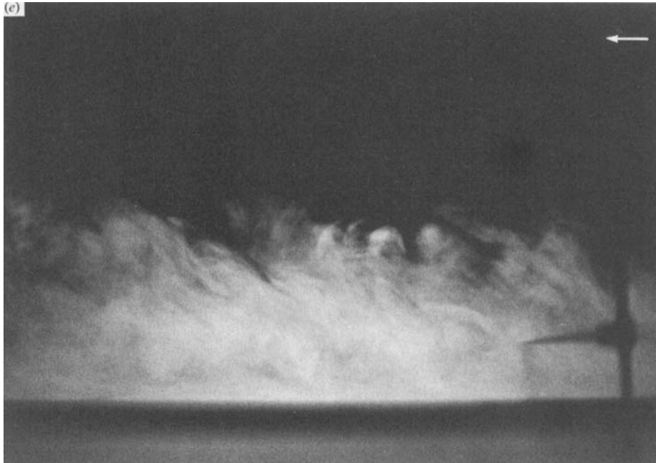
FIGURE 11. (a) Boundary layer approaching single-plate manipulator, l = 1.8\delta_m , h = 0.8\delta_m , Re_\theta = 1000 . (b) Manipulated boundary layer immediately downstream of single-plate device, l = 1.8\delta_m , h = 0.8\delta_m , Re_\theta = 1000 . (c) Manipulated layer approximately 25\delta downstream of single plate, l = 1.8\delta_m , h = 0.8\delta_m , Re_\theta = 1000 . (d) Manipulated boundary layer approximately 50\delta downstream of single plate, l = 1.8\delta_m , h = 0.8\delta_m , Re_\theta = 1000 . (e) Boundary layer immediately downstream of circular cylinder manipulator, D = 0.05\delta_m , h = 0.5\delta_m , Re_\theta = 1000 .
